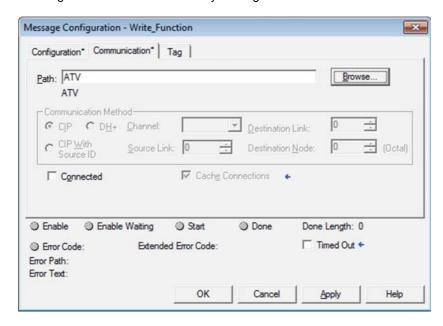
It is possible to read or write the ALL parameter by toggling the Read or Write bits.
