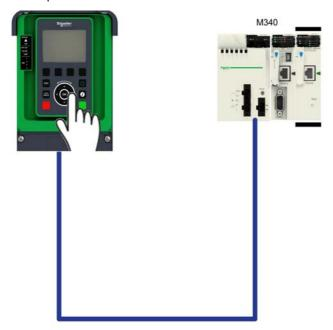
The drive is controlled from the communication but the reference value is adjusted on the display terminal. The control word comes from the controller and is written according to CiA 402 profile.
