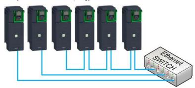
**NOTE:** In daisy chain topology, if one drive is turned off, an **[Fieldbus Com Interrupt]**  $\mathcal{L}$   $\mathcal{n}$   $\mathcal{F}$  error is trigged in the other drives connected to the same topology. To keep the integrity of Ethernet daisy chain network when one or more drives are powered off, add an external permanent 24VDc supply to the control block of the drive.
