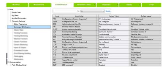
• Configure [Ref Freq 1 Config] F r I parameter to [Embedded Ethernet] E E H value.
