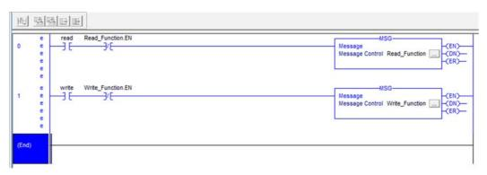
The Read Boolean will trigger the Read\_Function to read the # [ parameter.
