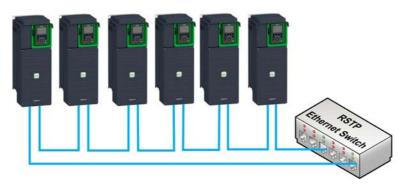
• Redundant ring topology with RSTP (with a RSTP
