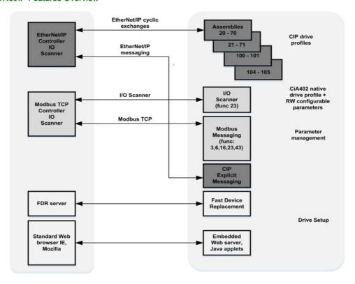
NOTE: When using ModbusTCP, it is advisable to use function codes 16 or 23 to control the drive.
